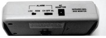
Side view of unit showing AC adaptor plug and switches to the alarm to Local or Remote and specify signal should sound as chime or alarm.
